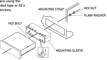
TYPICAL FRONT-LOAD DIN MOUNTING METHOD
